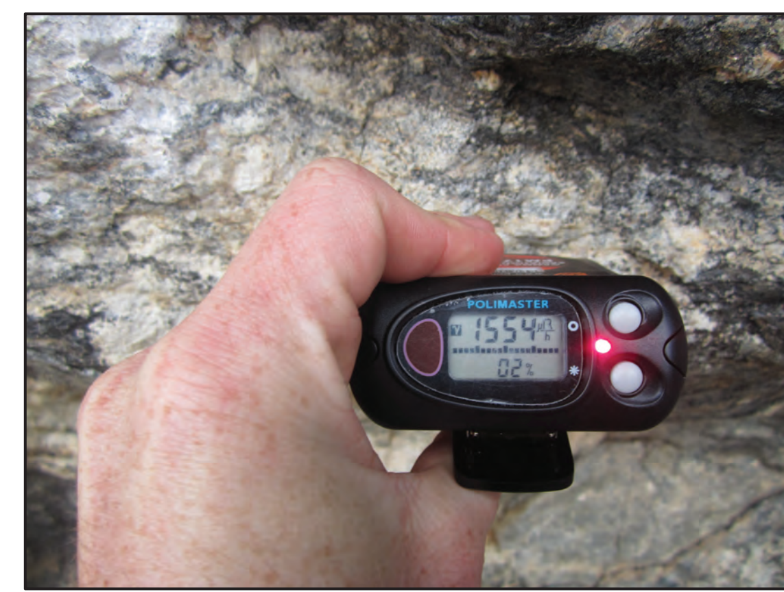
Figure 3: (above) Field relationships of 1) Pinto Gneiss, 2) Gold Park Diorite and 3) pegmatite veins at A) main U-Thor deposit and B) a prospect pit located ~300m east of main U-Thor deposit. (below) Use of radiation detector in field to locate ore rock
